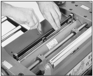
Figure 20. Tightening knives in cutterhead.
